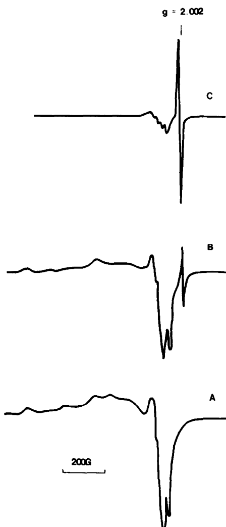
FIG. 1. EPR spectra of Cu(15)Y and effect on furan adsorption at 25°C. (A) Evacuation at 200°C for 4 hr. (B) Furan on Cu(15)Y. (C) Additional furan added to B.
